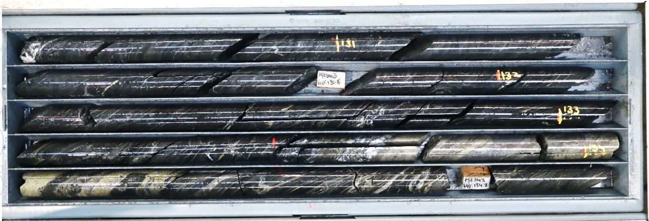
Figure 4. MZS43 133.5 – 134.5m. 1.0m of massive jamesonite (Sb sulphide) - chalcopyrite (Cu sulphide) - pyrite - arsenopyrite – tetrahedrite (Ag sulphide) mineralisation (Hanging Wall Lode).
