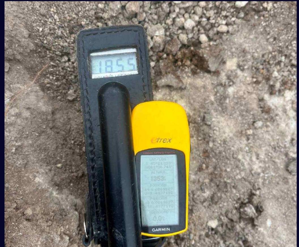
Elevated radioactivity at surface (measured in counts per second using an Exploration GR-110 tool) at recent site visit in May 2025
