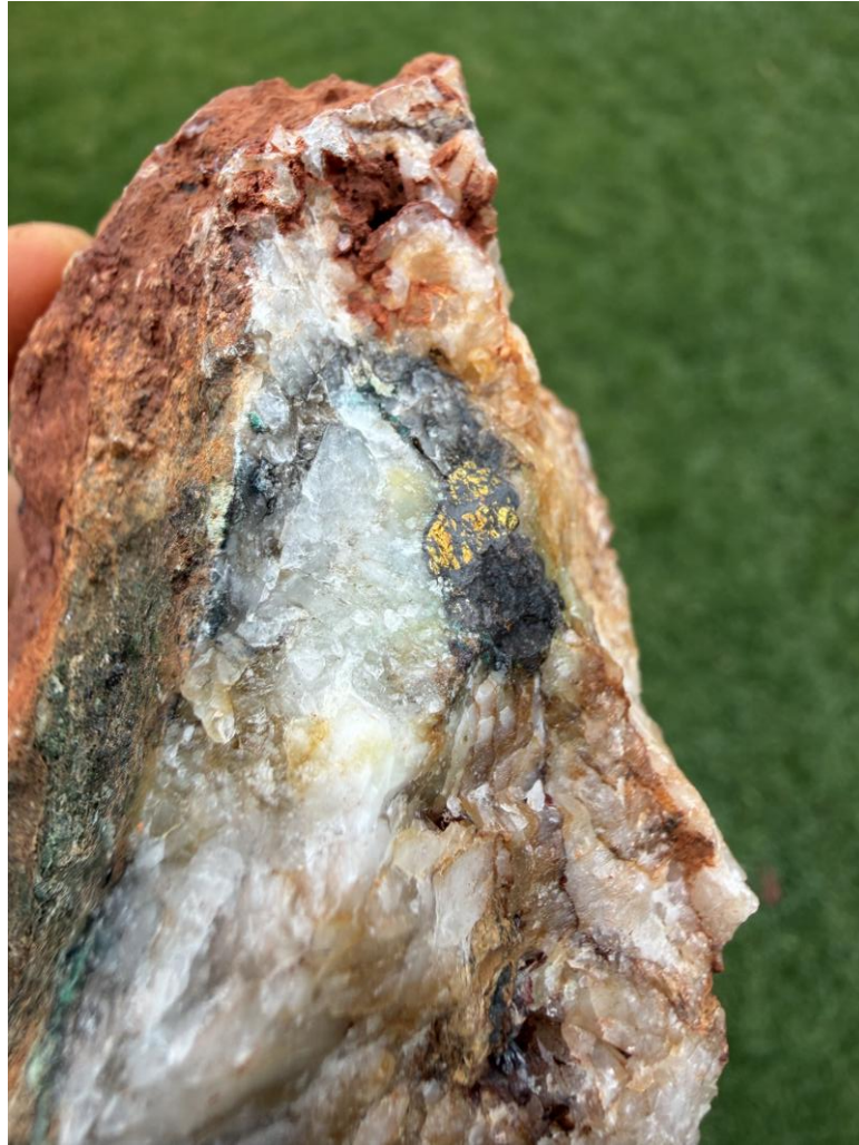
Figure 3: Close up of sample from GS000549 showing Malachite and Chalcopyrite
