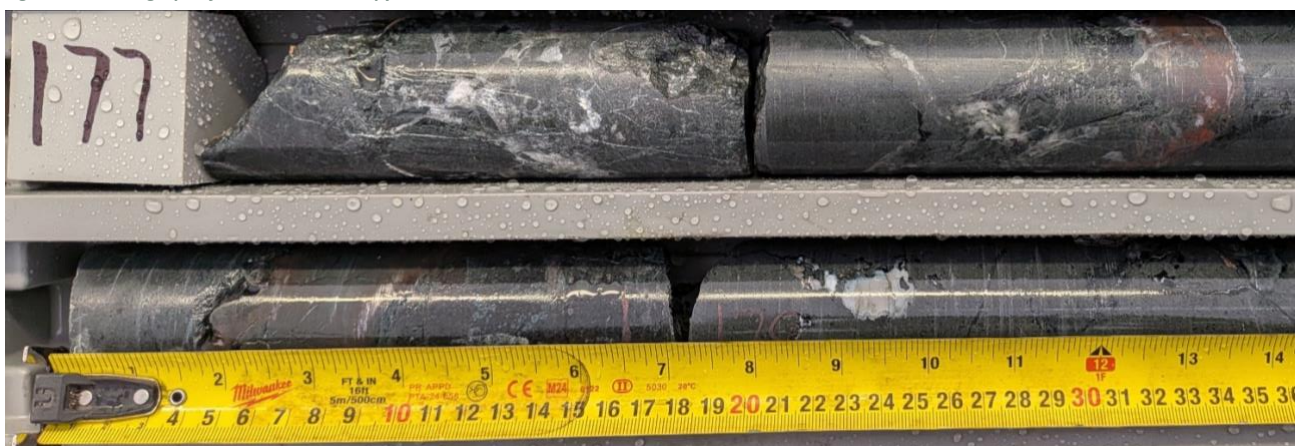
Figure 03 - Disseminated chalcocite within vein and breccia intervals in DAN26050 between 179-178m downhole.
