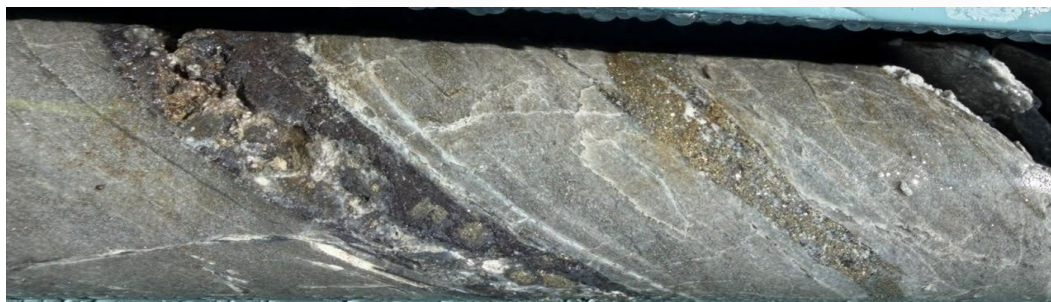
Figure 3 – Selected core photos showing vein sets with sulphides (pyrite, sphalerite, galena, +/- chalcopyrite), quartz +/- carbonate, +/- sericite, +/- clay minerals. (a) Section of sheeted vein set W1 (WWDT010, 113.25m) (b) Section of sheeted vein set W2 (WWDT010, 121.1m).
