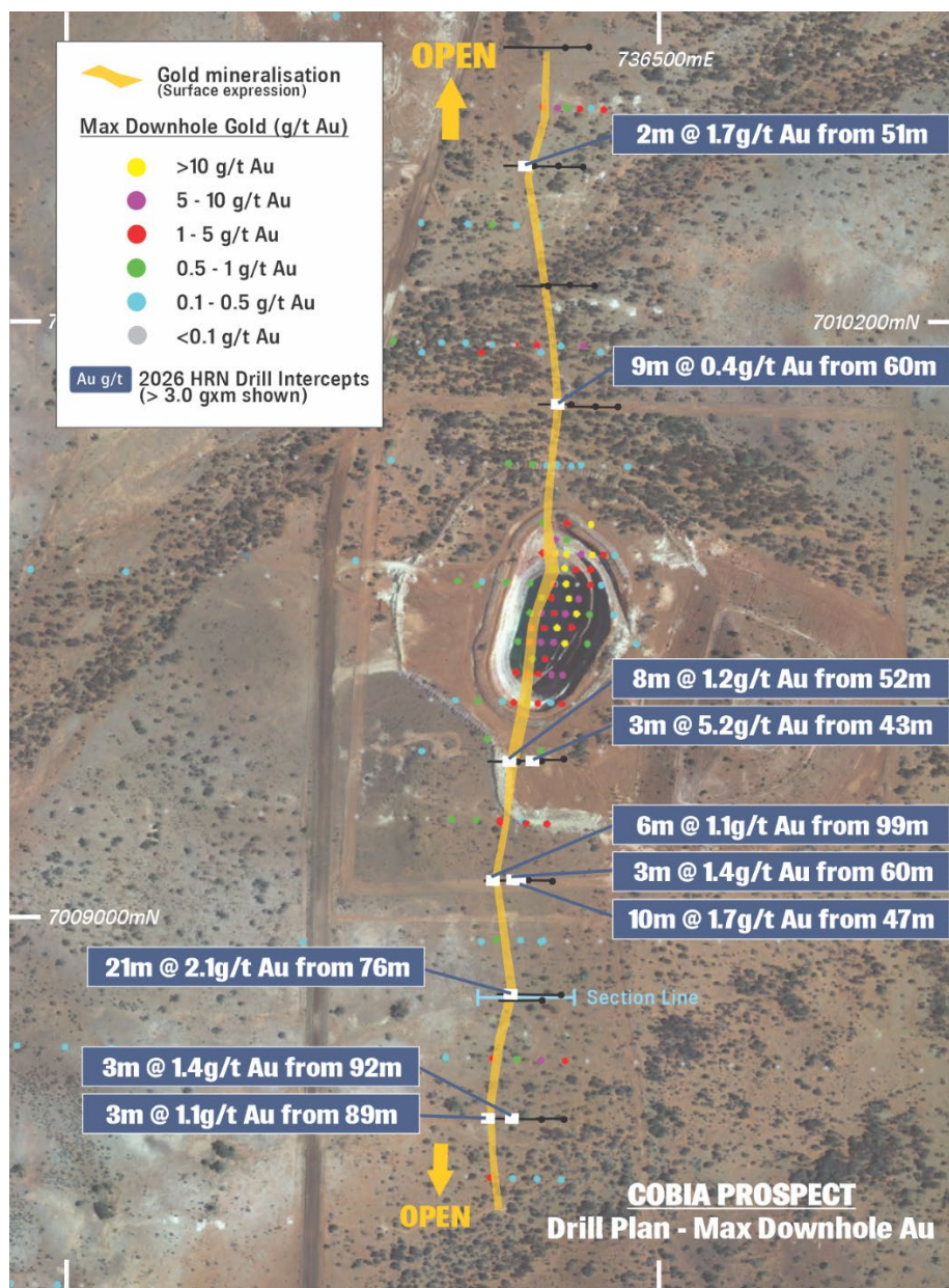
Figure 4: Cobia drill hole plan showing all drill collars coloured by max. downhole gold and recent intercepts over satellite image.
