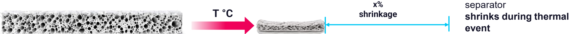
Conventional PE/PP separator base film
