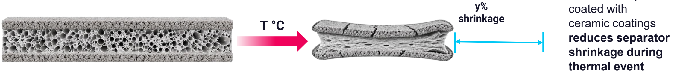
Ceramic coated PE/PP separator base film
