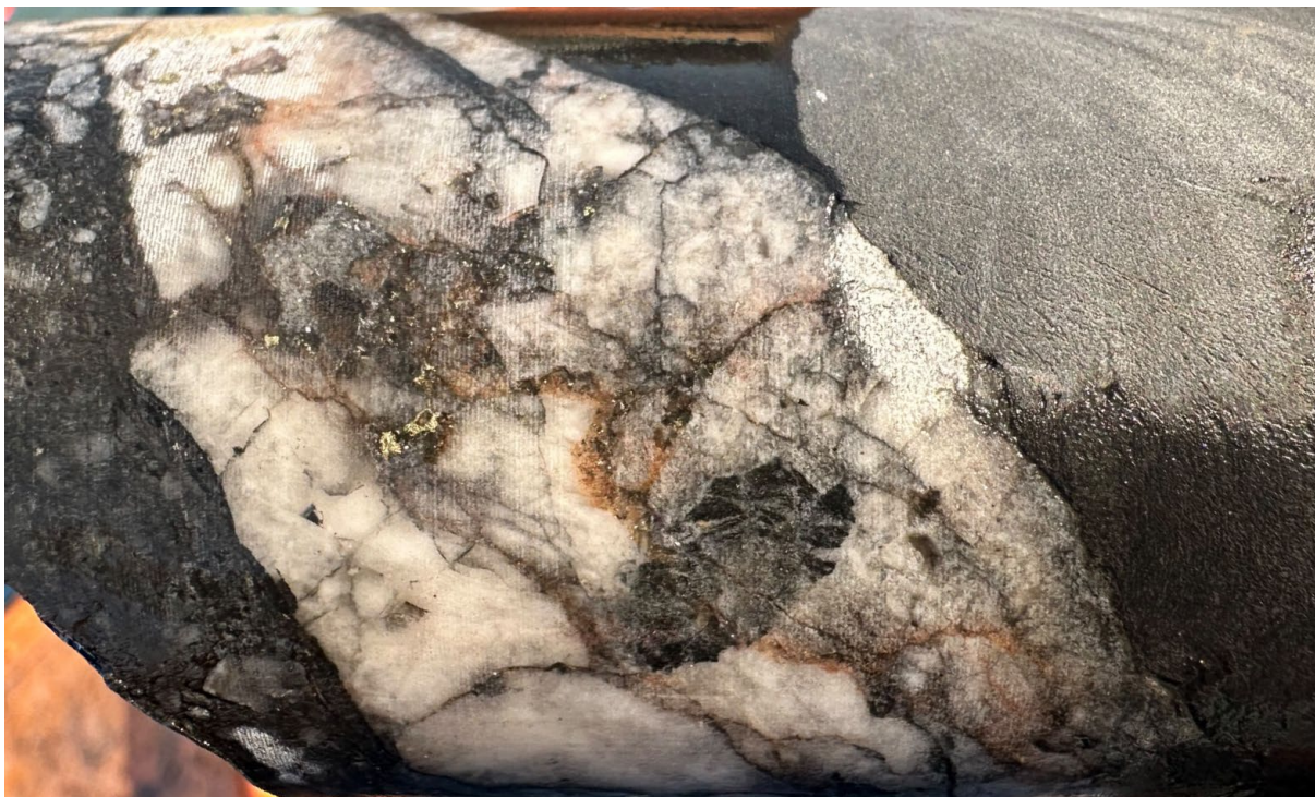
Figure 2: MD004DD NQ3 core at 593.85 m showing a thin (5 cm) quartz vein with ~1% disseminated chalcopyrite mineralisation and fragments of brecciated wall rock.
