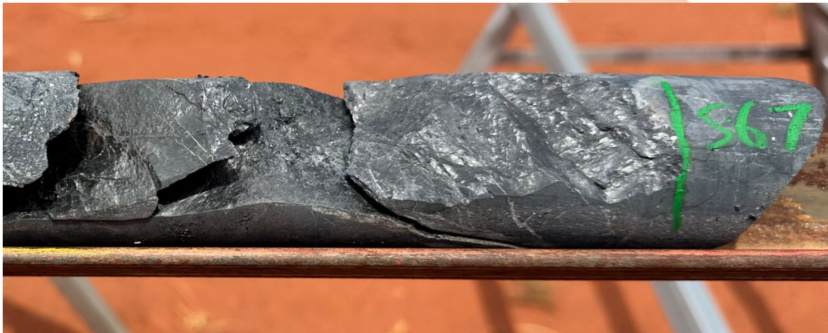
Figure 1: MD004DD NQ3 core (core is 45 mm width) at ~567 m depth showing dark, fine-grained, metasedimentary lithology with graphite developed along fractures and shear planes. This unit was intersected (with variably developed graphitisation) from ~505 m to 627.20 m downhole and provides an explanation for the conductor targeted by the drillhole.
