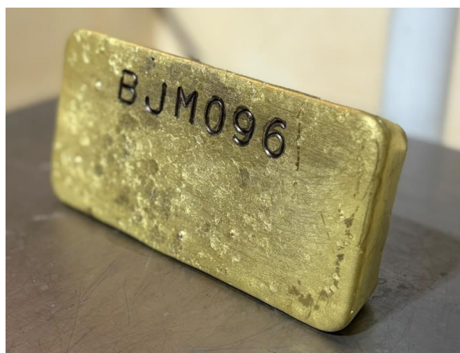
Figure 6: Gravity doré bar BJM096 from the 15 September 2026 smelt (76.8% gold assay)
