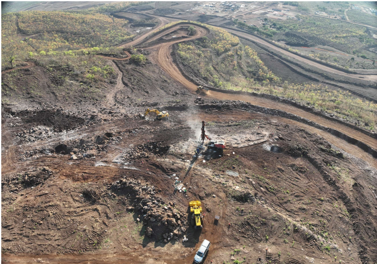
Picture 10. Development of the upper pit access ramp and drilling activities progressing to open additional mining faces at Kangankunde
