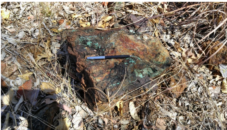
Figure 3a. A photo of rock chip SampNo 102147 collected from the Windmill area of EPM 25970 (Table 1) assaying 0.33 g/t Au and 10.7% Cu. Figure 3b. A photo of the sawn mullock rock chip SampNo 102147. Both photos show visible copper oxide mineralisation.
