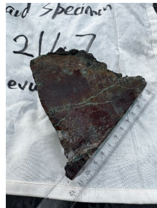
Figure 3a. A photo of rock chip SampNo 102147 collected from the Windmill area of EPM 25970 (Table 1) assaying 0.33 g/t Au and 10.7% Cu. Figure 3b. A photo of the sawn mullock rock chip SampNo 102147. Both photos show visible copper oxide mineralisation.
