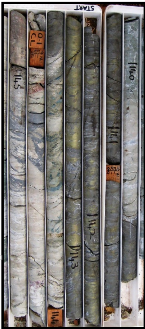
Figure 6a. Photo of marked out diamond drillcore from hole OK07DD18 prior to sampling, showing the massive sulphide pyrite-chalcopyrite-sphalerite lens assaying 4m @ 5.91% Cu, 3.64% Zn, 0.55 g/t Au and 13.6 g/t Ag from 140m to 144m depth downhole drilled below the floor of the underground workings at OK Mine.
