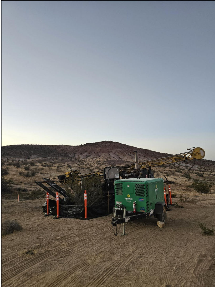
Figure 2: Rig mobilised onto the first drill collar position.
