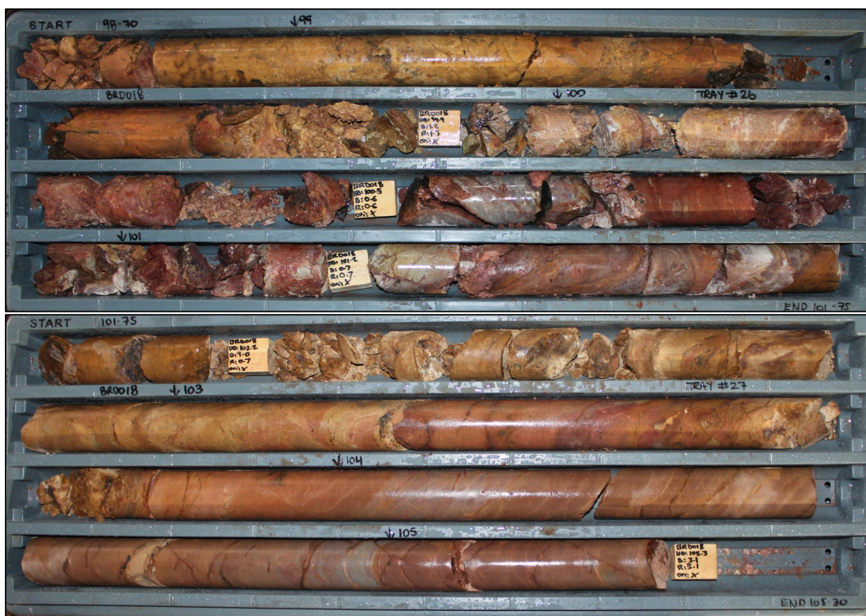
Figure 4: Historic BRD018 core showing the newly assayed oxide interval of 3m at 2.0g/t Au & 14g/t Ag from 99m, including 1m at 4.2g/t Au & 12g/t Ag from 100m.
