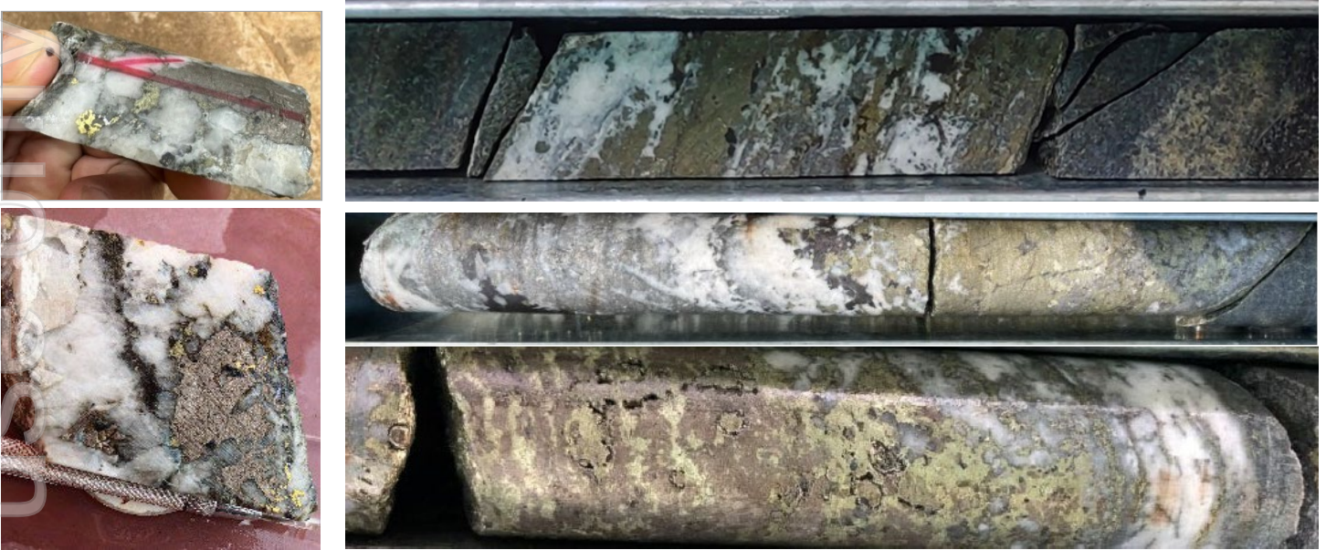
Figure 6 | Mineralised veins in Memot diamond core. Quartz veining with pyrite, arsenopyrite, pyrrhotite, chalcopyrite and sphalerite sulphides. In order from left photographs: DD24MMT243 - 1m @ 2,090.00g/t Au from 130m. Right photos from top to bottom DD21MMT001 - 1m @ 8.91g/t Au, 2.16% Cu from 48m, DD22MMT013 - 0.4m @ 17.70g/t Au, 230g/t Ag, 2.78% Cu, 0.56% Pb and 1.74% Zn from 190m and DD21MMT006 - 1m @ 25.4g/t Au, 73g/t Ag, 1.81% Cu, 0.1% Zn from 30m
