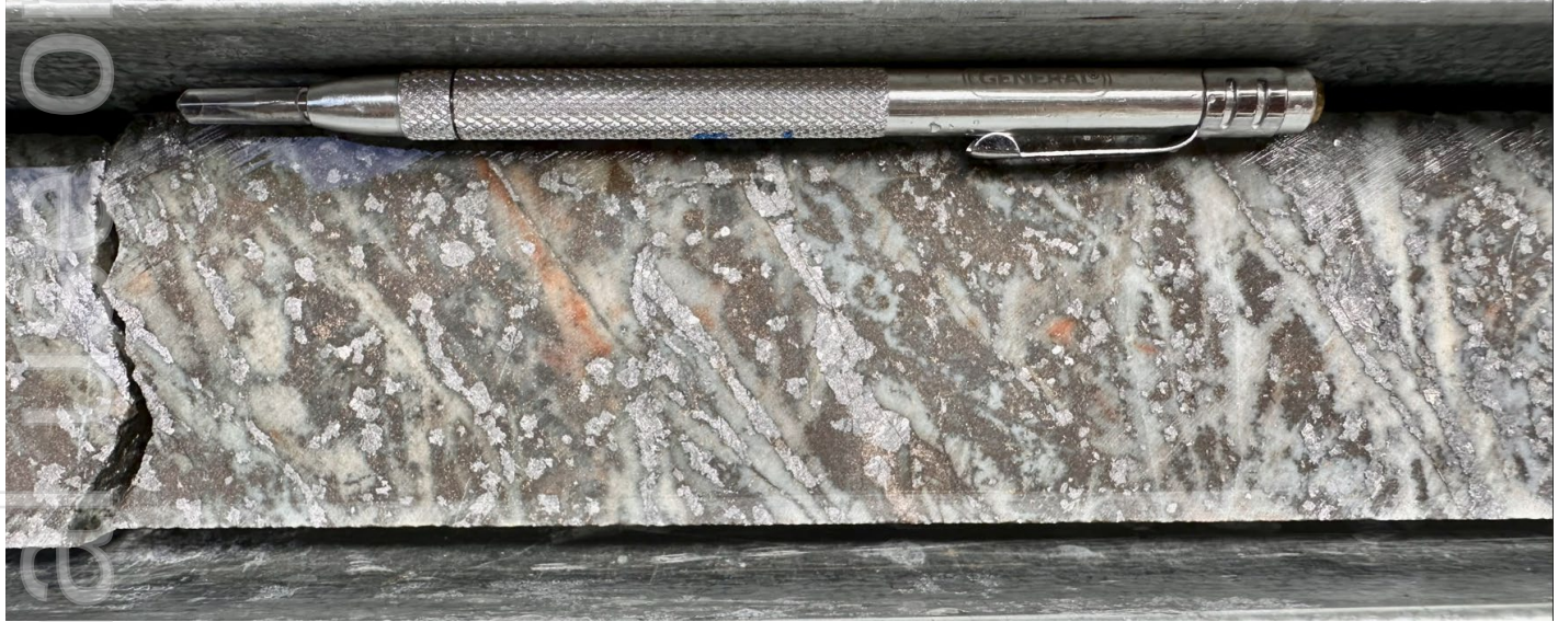
Figure 2 | Mineralised vein in RCDD26OKV824W1 at approximately 530.5m downhole depth. The vein comprises predominantly euhedral arsenopyrite associated with quartz carbonate veins within a hornfelsed sedimentary host. The photograph shows approximately 20cm of core from within the intercept of 78.80g/t Au from 530–531m
