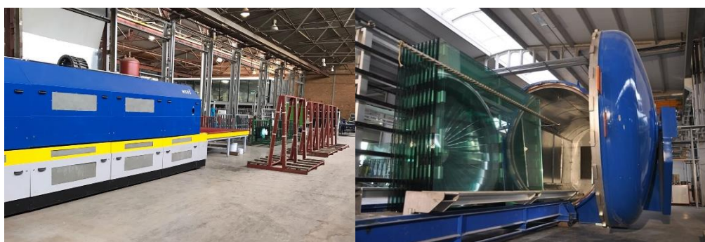
Some of Glass Partners' manufacturing facilities – toughening furnaces and glass laminating autoclave.
